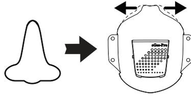
Press down on top portion of face mask to increase the nose bridge width.
