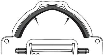
Stick the top sponge at nose piece to prevent air leak from above nose area.
