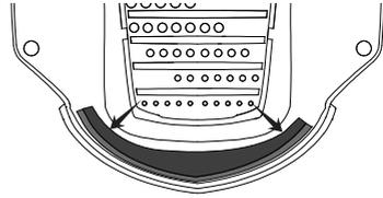
(Optional) you can stick the sponge on the bottom of the mask as indicated in the picture above to prevent air leak.
